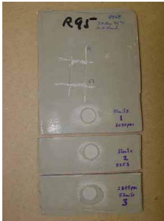
Adhesion Panel; NACE RP0394-2002 30 Day/203°F H 2 O Soak and ASTM D 4541-02 Test After the 30 Day/203°F H 2 O Soak
