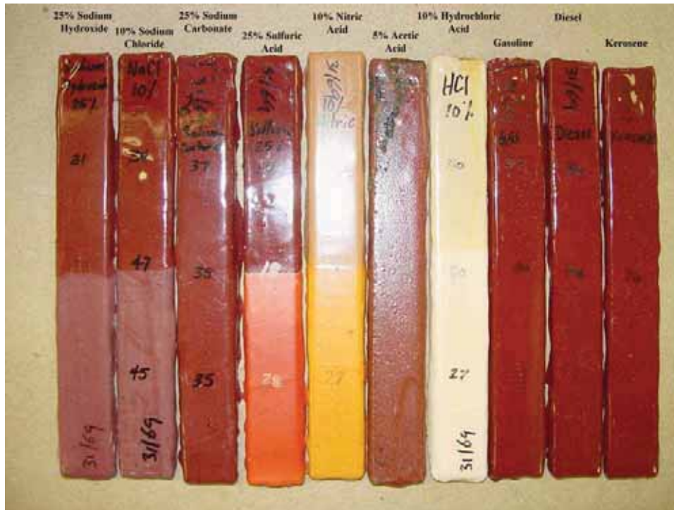
Chemical Resistance Panels; ASTM G 20-88
