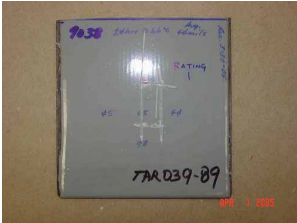
Hot Water Soak Panel; NACE RP0394-2002 (24 Hours @ 150±5°F / 66±3°C)
